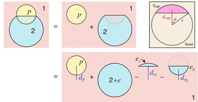
**Fig. 2** A cartoon depicting the initial particle drop system split into a series of different domains to facilitate the calculation of the centre of mass of the system. Inset: A spherical cap with volume  $v_{cap}$  and centre of mass  $d_{cap}$  formed by taking a portion of a sphere of radius  $r$ , with subtended angle  $\phi$ .
